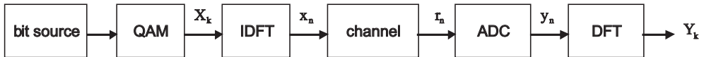
Fig. 1.5: System model showing the transmission over one subchannel in the OFDM system with ideal synchronization
